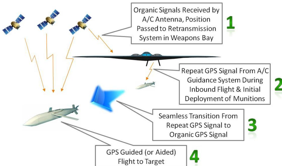
**Figure 2. GPS Retransmission System Function in Aircraft Deployed Munitions**
